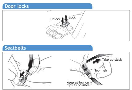
If belt is fully extended, then retracted even slightly, it cannot be re-extended beyond that point, unless fully retracted again. This feature is used to help hold child restraint systems securely.
